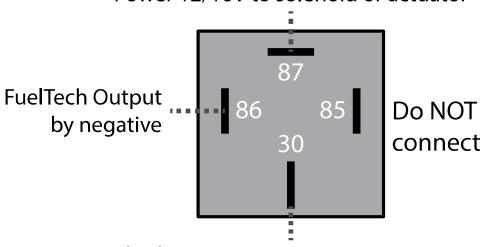
Switched Power 12/16V, minimum 30A circuit (relay bottom view)
